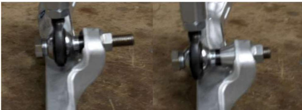
4. Install one end link into the sway bar. As shown in the images on the next page, make sure both rod ends are in the middle of their articulation, and the end link is as close to perpendicular to the ground as possible. When installing the new SPL Parts end links, you should not have to apply any force to the control arm or the sway bar to install the
