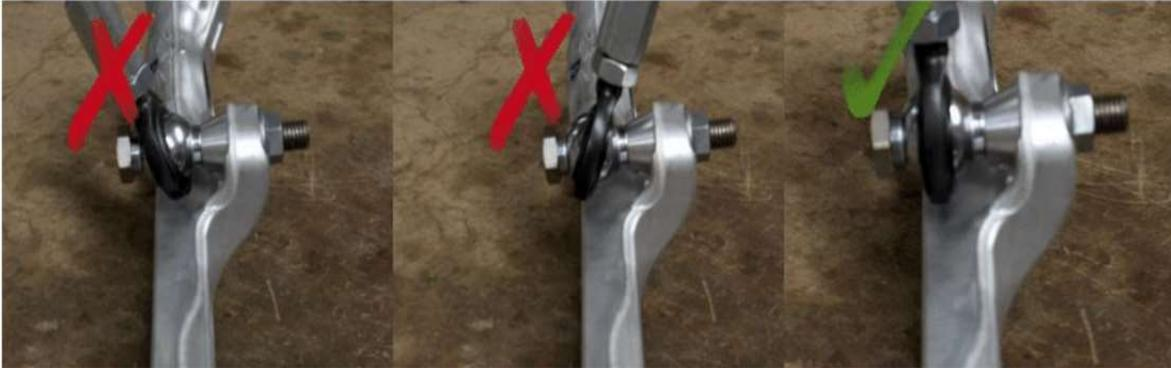
5. Install the other end link into the sway bar. Adjust the length of this end link so you do not have to apply any force to the sway bar or control arm to install the stud. As shown in the images below, the stud should line up well and slide through easily. If you are unable to achieve this, change the length of the end link on the other side of the vehicle and try again.
